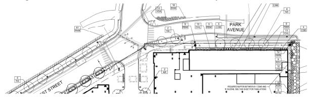
Diagram above is extracted from the Founders Row landscape drawing. It shows sewer lines, electrical lines run along Park, about 2 ft. from the street curb. (Shown as grey lines.) This means that trees have to be planted at least 7 ft. from the curb. These utilities run down the length of Park.
